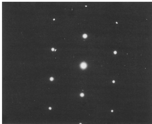
Figure 11 STEM electron-diffraction. Selected area diffraction pattern from one of the Cr 2 N precipitates.
