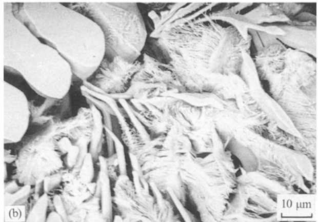
Figure 6 CrN precipitates; different morphologies. (a) The three-dimensional features of the different chromium nitrides after removal of the austenitic matrix by etching with bromine alcohol solution. (b) Three different microconstituents are shown: (i) in the upper left are primary dendrites formed during cooling; (ii) the larger linear precipitates are CrN-austenite eutectic phase formed during final solidification; (iii) the fine lamellar precipitates are Cr 2 N-austenite "false pearlite" formed from solid-solid transformations.
